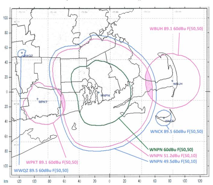
As defined in FCC DA 10-208 / MM Docket No. 99-325, there is contour overlap between WNPN's 89.3FM's 51.2dBu interfering contour and with WPKT 89.1 and WBUH 89.1's 60dBu service contours. Therefore, WNPN is limited to -14dBc HD Radio digital injection on the lower sideband.
