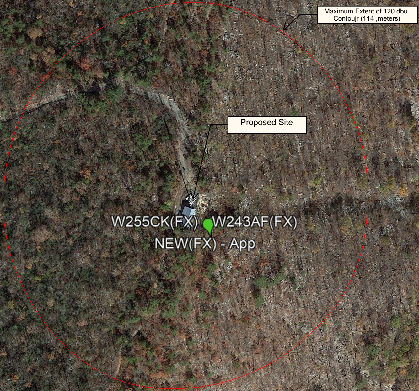
Exhibit 13 Figure 3 Extent of interfering contour New FM Translator, Front Royal, VA Winchester Radio Broadcasters, LLC
