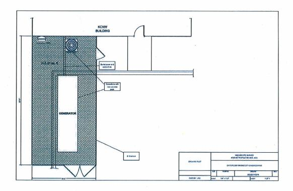
Plus a right of way for Entercom to bury cables from the Tower to the transmitter room.
