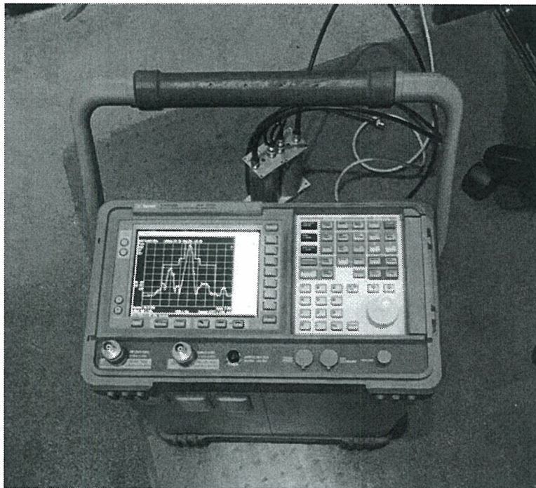
Agilent E4402B Spectrum Analyzer used for measurements
