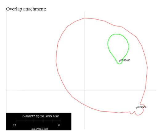
Red contour: K246CL, BPFT-20160729AAX – 40 dBu interference contour Green contour: K300DC, BPFT-20160728AHP – 60 dBu protected contour
