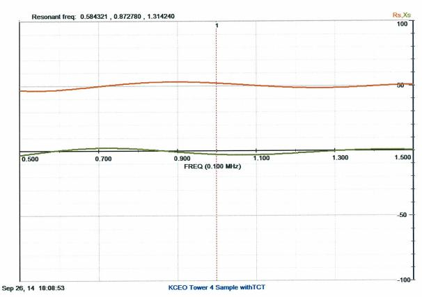
Impedance of Tower 4 line at 1000 KHz, monitor end with transformer connected at other end:
