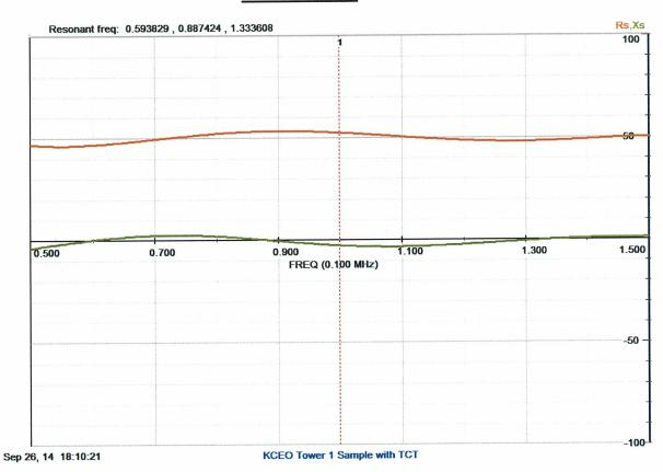
Impedance of Tower 1 line at 1000 KHz, monitor end with transformer connected at other end:
