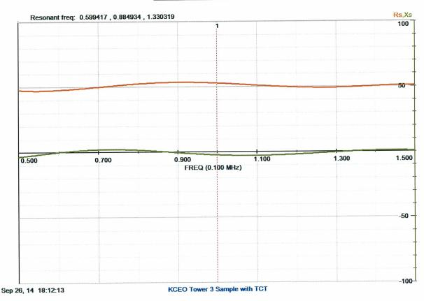
Impedance of Tower 3 line at 1000 KHz, monitor end with transformer connected at other end:
