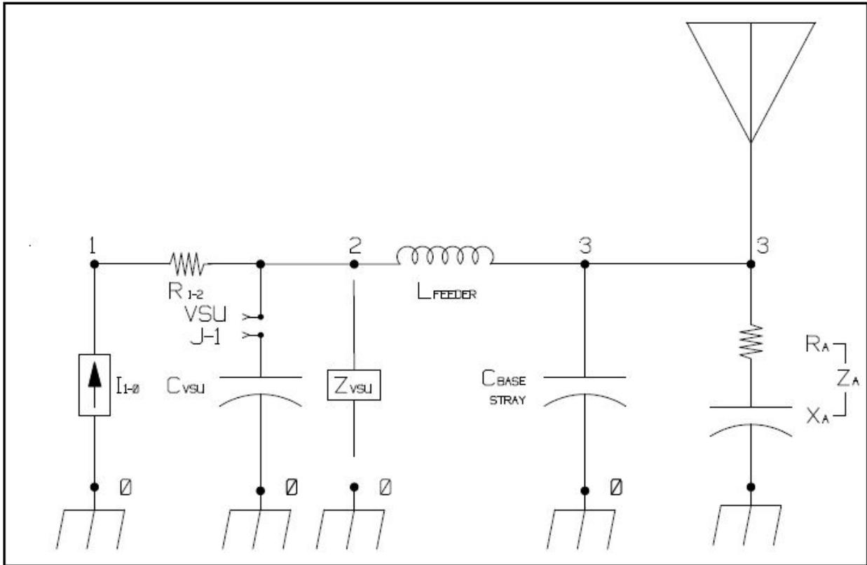
**The base insulator, Austin Xfmr & Isocoupler capacitances are lumped at Node-3**
