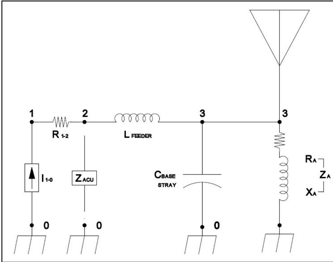
**The base insulator & other stray capacitances are lumped at Node-0-3**
