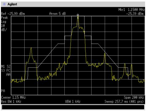
Several adjacent channel stations can be seen and all were identified. The signal at 1220 kHz is an intermod mix of 2 X 1150 – 1080. It is 62.9 dB below KXET.
