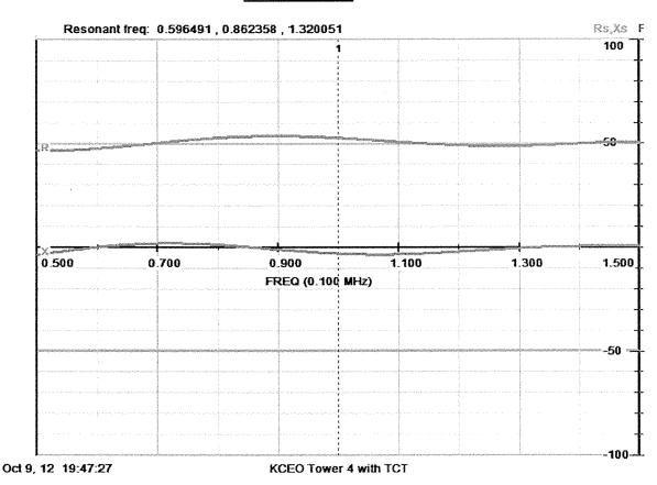
Impedance of Tower 4 line at 1000 KHz, monitor end with transformer connected at other end:
