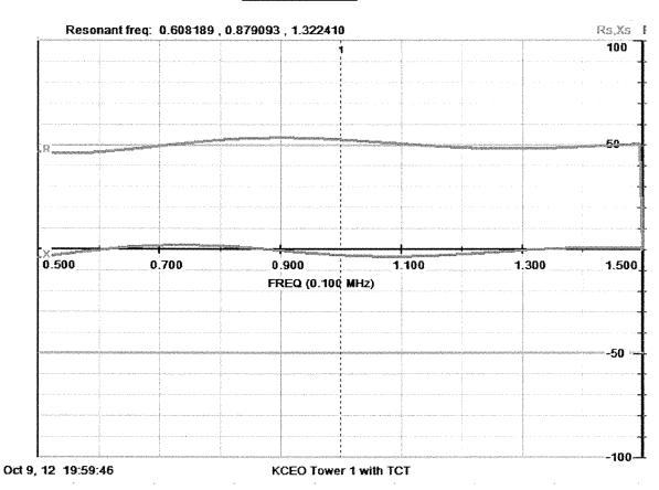
Impedance of Tower 1 line at 1000 KHz, monitor end with transformer connected at other end:
