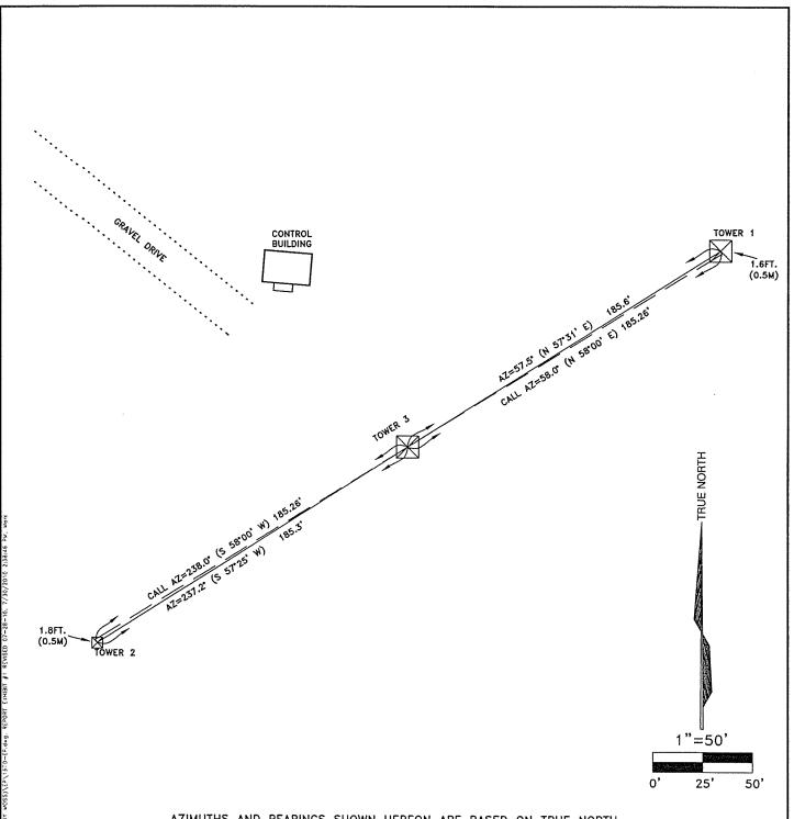
AZIMUTHS AND BEARINGS SHOWN HEREON ARE BASED ON TRUE NORTH DISTANCES SHOWN ARE SURFACE MEASUREMENTS
