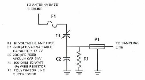
KPTK-AM Custom Capacitive Voltage Divider Antenna Sampling System
