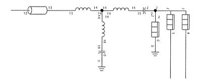
Nodes 3 and 4 above connect to the other three towers and represent the calculated mutual impedances to/from each tower from the matrix.
