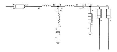
Nodes 3 and 4 above connect to the other three towers and represent the calculated mutual impedances to/from each tower from the matrix.
