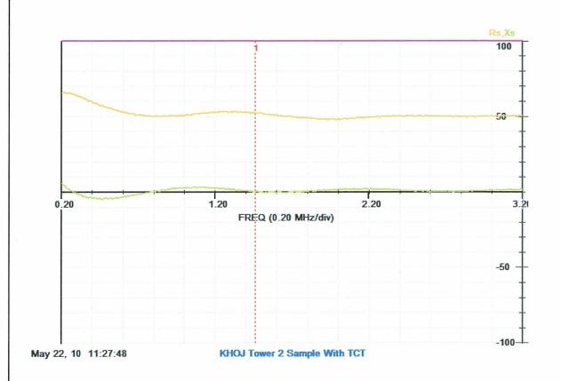
Impedance of Tower 2 line at 1460 KHz, monitor end with transformer connected at other end:
