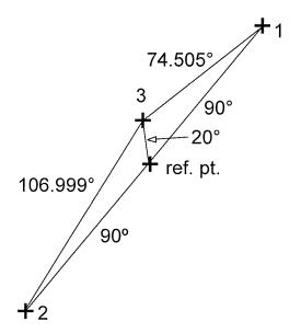
A copy of the survey report is attached. This corresponds to a maximum relative spacing error of less than  $+0.1^{\circ}/-0.22^{\circ}$  and bearing error of less than  $+0.0^{\circ}/-0.13^{\circ}$ , well within the allowed tolerances of  $+/-1.5^{\circ}$ .
