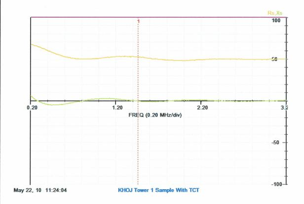
Impedance of Tower 1 line at 1460 KHz, monitor end with transformer connected at other end:
