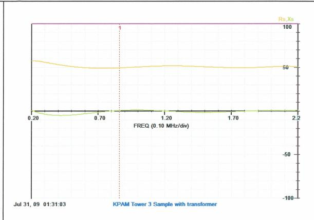
Impedance of Tower 3 line at 1460 KHz, monitor end with transformer connected at other end:
