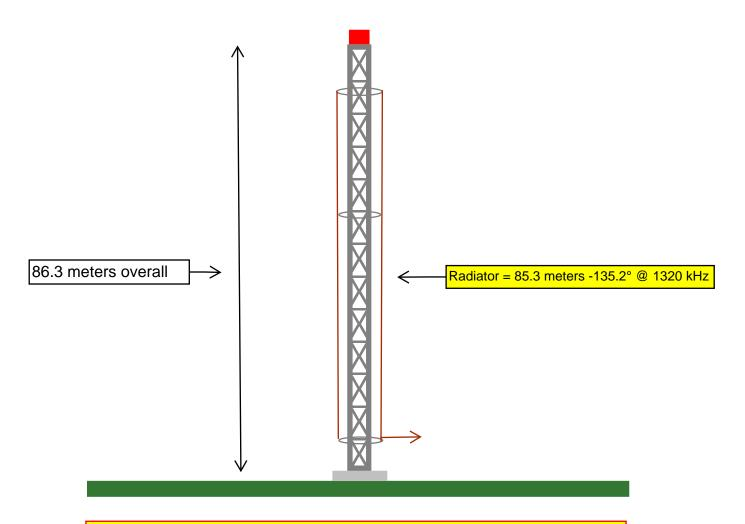
WVNZ will be combined with WHAN on 1430 kHz, 1 kW Day into its existing 85.3 meters radiator which is 135.2° @ 1320 kHz. The efficiency at 1320 kHz was calculated using the Commissions Figure 8 tool to be 332.2 mV/m/km/kW based on the existing 120 radial 52.4 m ground system
