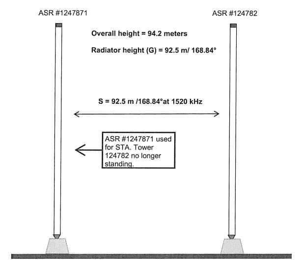
WBZW 1520 kHz to be diplexed with WRSO(AM) on 810 kHz. Existing ground system is equivalent to a full 90 degree system at 1520 kHz.
